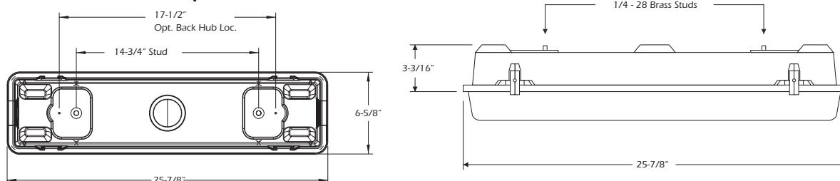
Note: Brass Studs on Inside of Unit are 10-32
