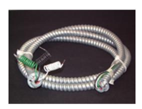
All Whips will be supplied with 6" End Leads on both ends. A number 8 terminal ring on one end of the green ground which is standard for easy installation. Whips are supplied in 3 wire, 4 wire, and 5 wire.
